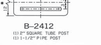
B-2412 (1) 2" SQUARE TUBE POST (1) 1-1/2" PIPE POST
